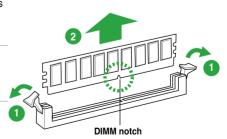
2 Remove the DIMM from the socket
